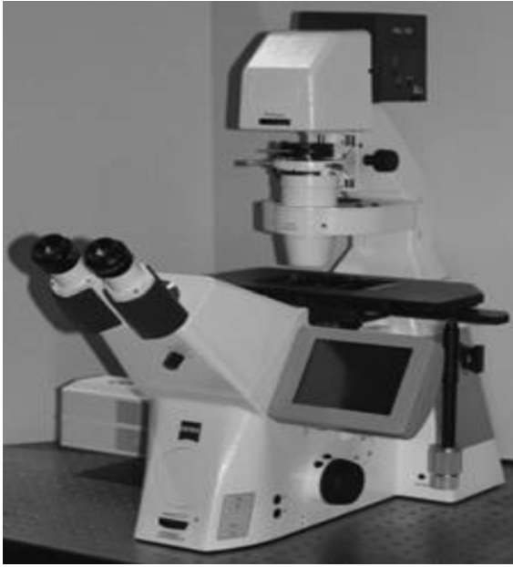
Fig. 3. Axio-observer inverted motorized microscope used to image RBCs in whole blood smears for different glucose concentrations [35].
